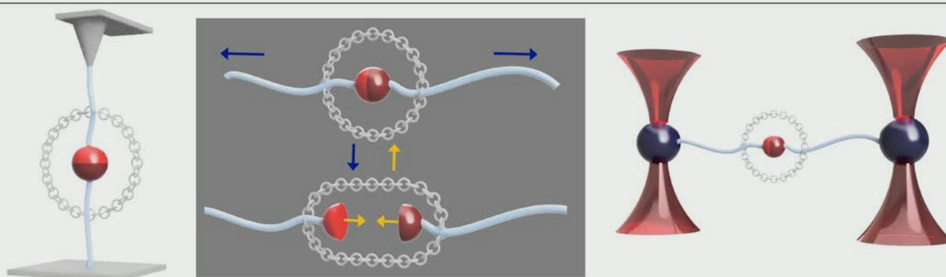
**Figure 1:** Schematic of the general objective of ChemForce. The concept of tethered bonds is shown in the central part. The partners of the bond stay in close proximity after being broken open and can rebind. Single-molecule force spectroscopy by AFM (left) or OT (right) is used to monitor the process in various environments (solvent, pH, presence of reagents, competitors, stimuli, ...).
