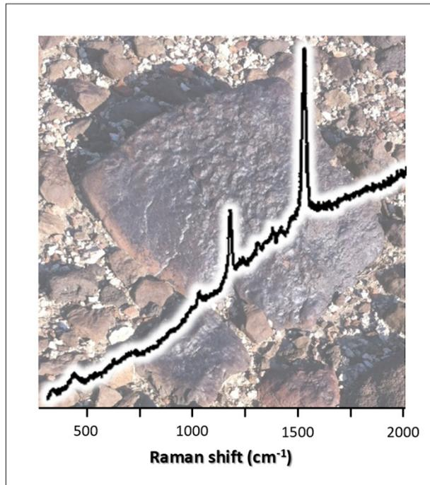
Figure 6. Desert varnish from Death Valley, California and a Raman spectrum of carotenoid detected at (1005, 1150 and 1510  $\text{cm}^{-1}$ ) is association with quartz (detected at 465  $\text{cm}^{-1}$ ) within the mineral coating
