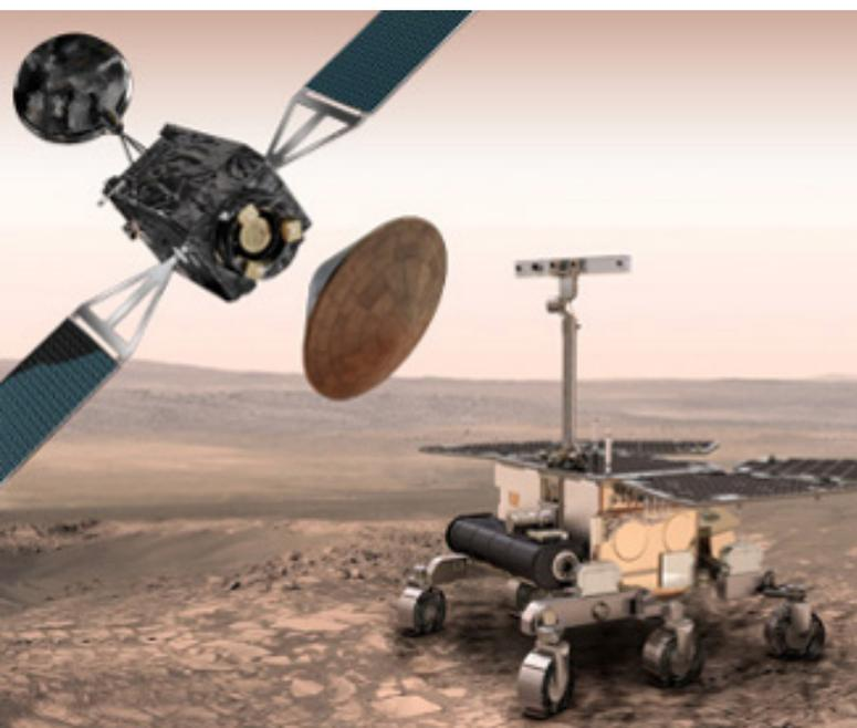
Figure 2. The ExoMars mission (ESA/Roscosmos) with the Trace Gas Orbiter (TGO), the *Schiaparelli* lander and the ExoMars rover (credit ESA)
